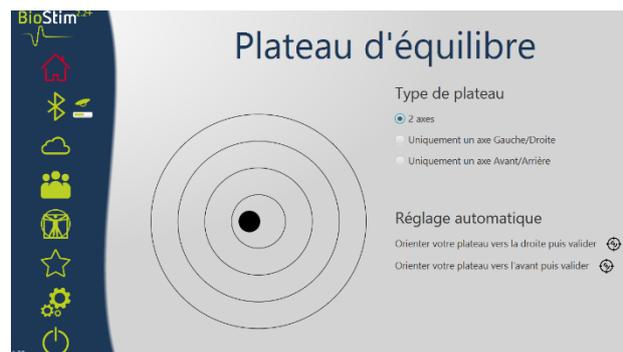
Note: During adjustment, the movement of the dot on the target may be reversed. After adjustment, the movement of the stage should cause the dot on the target to move in a consistent manner.
