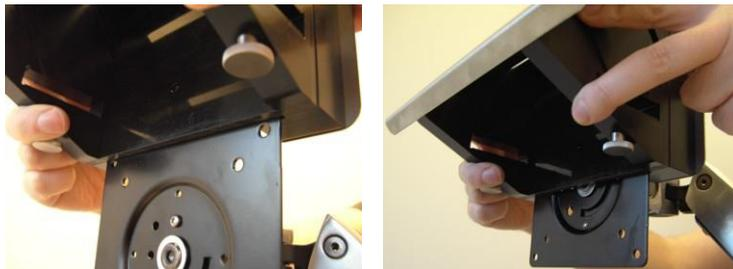
*Figure 3-10. Inserting the Handpiece Tray onto its Base*
