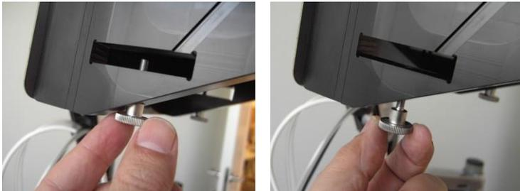
*Figure 3-18. Releasing the Cup Holder's Thumb Screw*
