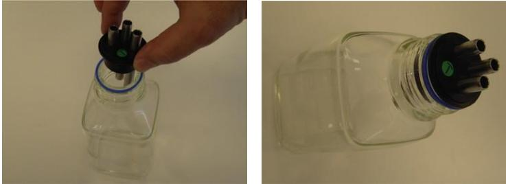
*Figure 3-33. Inserting the Stopper into the Jar's Neck*
