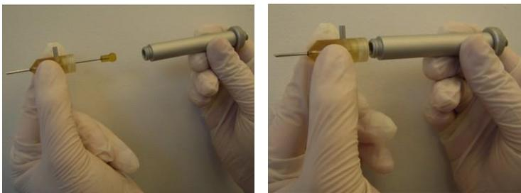
*Figure 3-79. Connecting the Head to the Handpiece Body*
