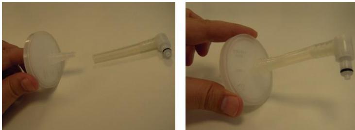
*Figure 3-39. Connecting the Long Tube and Fitting to the Filter's Inlet Port*
