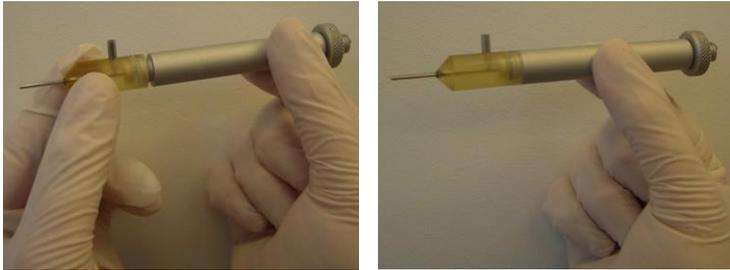
**Figure 3-80. Screwing the Head to the Handpiece Body**
