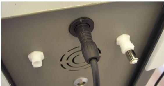
*Figure 3-68. Handpiece Cable Connected*
