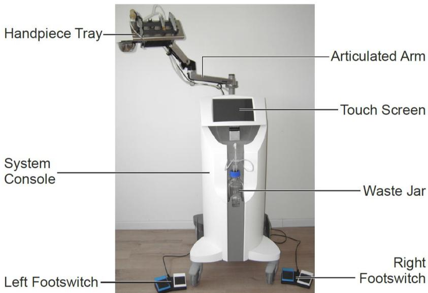
**Figure 4-1. System Components (Front)**
