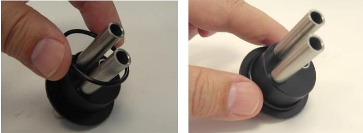
*Figure 3-31. Installing the Rubber Gasket on the Stopper*
