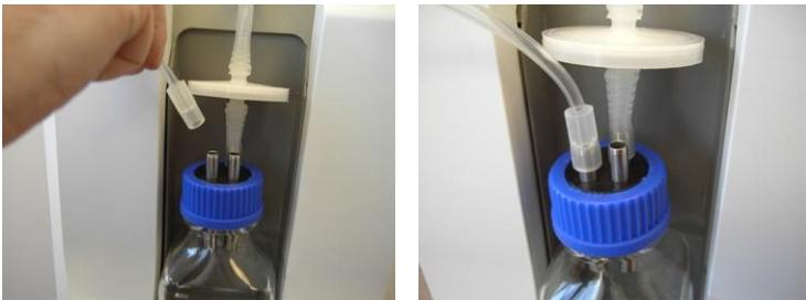
*Figure 3-61. Connecting the Extraction Tube to the Jar*
