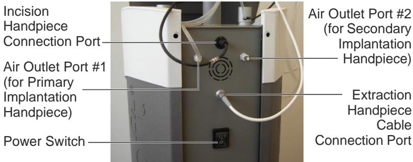
Figure 4-3. System Components (Upper Rear)
