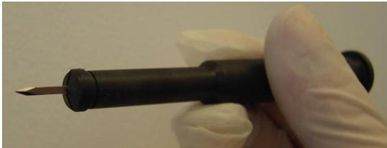
*Figure 3-70. Incision Blade Inserted into the Blade Holder*
