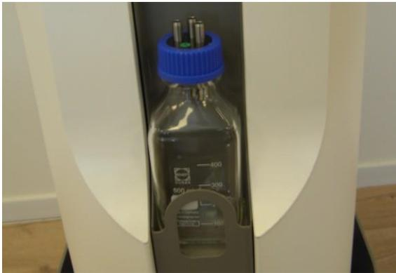
*Figure 3-36. Waste Jar Placed in its Housing on the System*
