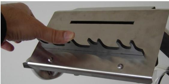
*Figure 3-15. Pushing the Lower Handpiece Holder in*
