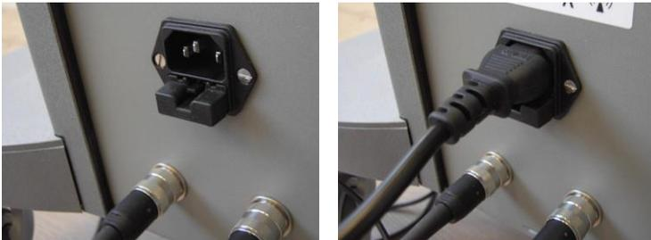
*Figure 3-92. Power Connection Port on the System's Rear Side*
