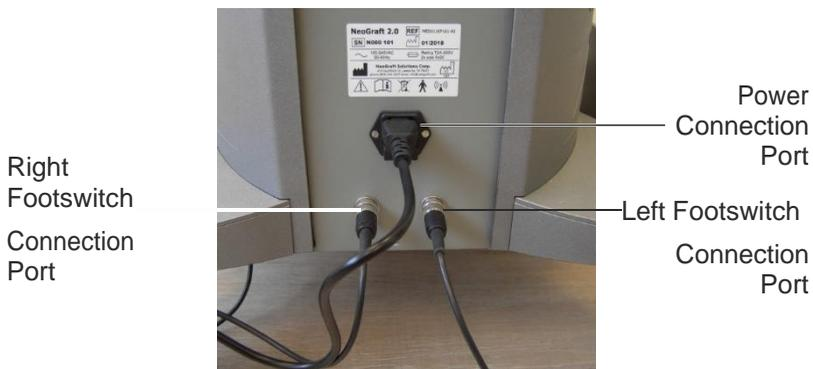
Figure 4-4. System Components (Lower Rear)
