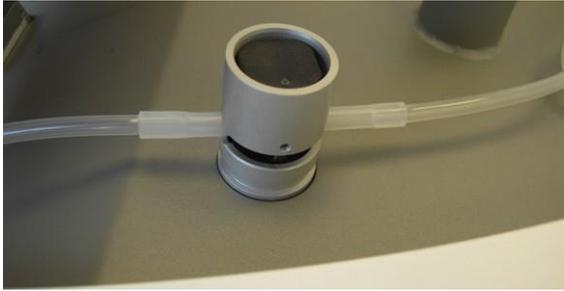
*Figure 3-90. Implantation Tube Inserted into the Right Electrovalve*
