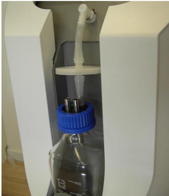
***Figure 3-44. Filter Assembly Installed***
