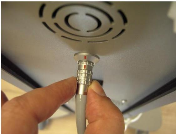
*Figure 3-46. Connecting the Handpiece Cable Connector*
