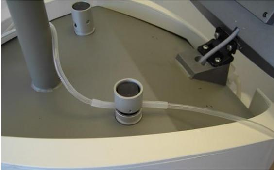
*Figure 3-65. Extraction Tube Inserted into the Left Electrovalve*
