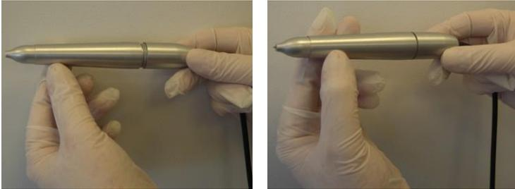
*Figure 3-73. Screwing the Handpiece Body to the Handpiece Base*
