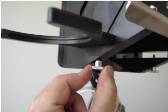
*Figure 3-20. Tightening the Cup Holder's Thumb Screw*
