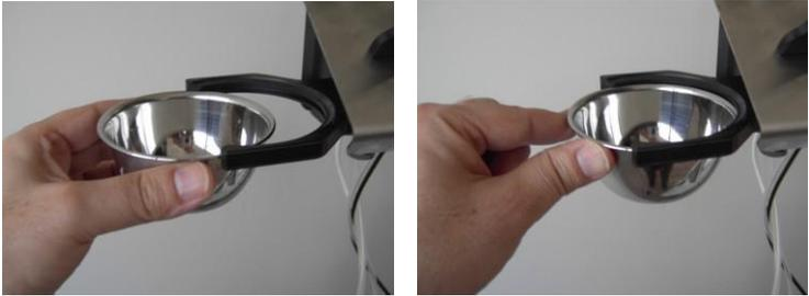
*Figure 3-21. Inserting the Cup into the Cup Holder*
