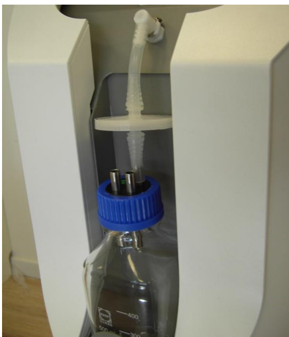
Figure 3-44. Ensemble de filtre installé
