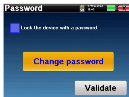
You can access the password configuration window later from the "Config" menu and then "System". This window allows you to change the password, but also to activate or deactivate the lock. If you forget your password, please contact Électronique du Mazet to receive an unlock code.
